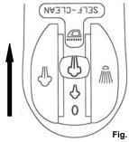
Steam is produced as soon as the iron is held in the horizontal position. Steam will stop coming out when the iron is put on its heel in a vertical position or by sliding the steam lever to "0".
